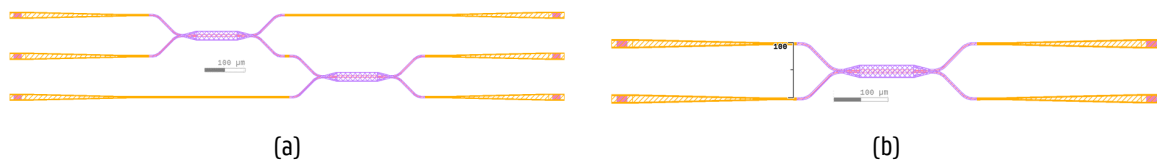
Figure 5.7: On (a), the design of an isolated node conformed by cascaded 2x2 MMIs is depicted. On (b), the testing 2x2 MMI is shown.
