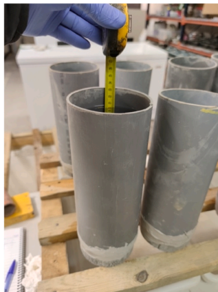
Fig. 2. Water permeability test setup.
