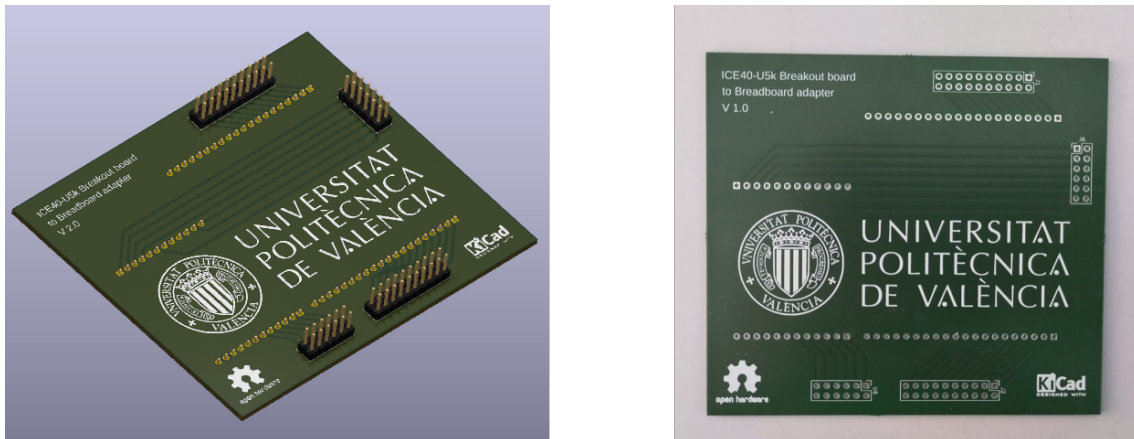
Figure 5.16: Kicad render of ICE40UP5K Breakout board to breadboard adapter and PCB Fabricated.
