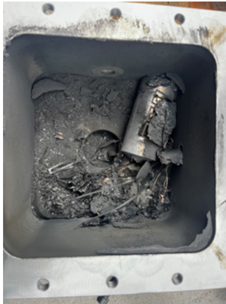
Figure 4.65 : 4695 cell at calibration test after TR
