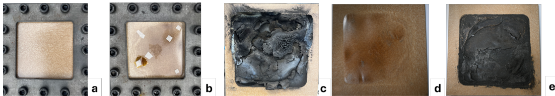
Figure 4.46 : GF/PPS 2 a) before TR (front), b) after TR (front), c) after TR (back), d) after TR and cleaning (front), e) after TR and cleaning (back)
