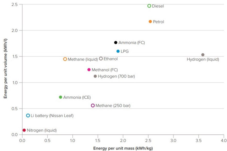
Figure 2.5: Specific energy and energy density for fuels [44]
