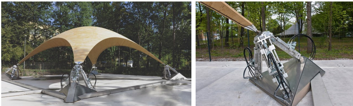
Figure 5. SmartShell experimental prototype with actuators integration on three supports at the University of Stuttgart campus in 2012.
