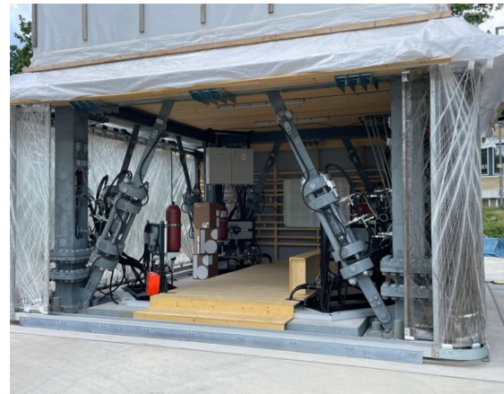
Figure 6. Demonstrator of the experimental prototype at the University of Stuttgart campus in 2021, and detailed view of the integration of actuators in a frame.
