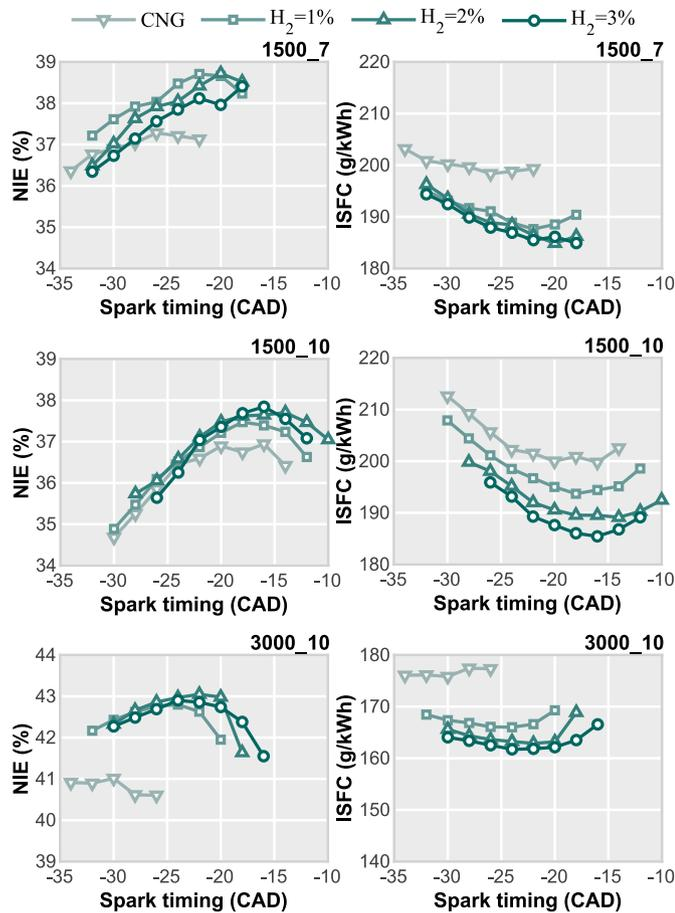
Fig. 4. NIE and ISFC for different hydrogen substitution percentages for different spark timing values.
