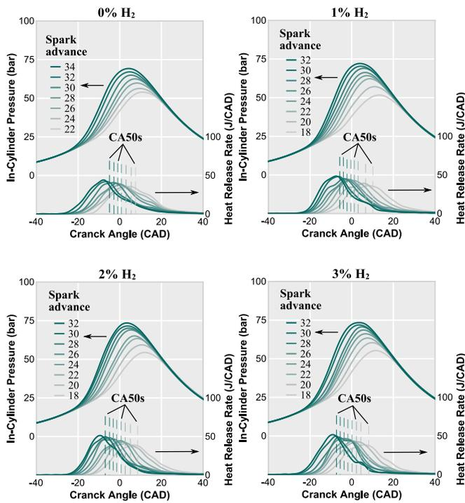
Fig. 2. In-Cylinder Pressure and HRR profiles for different hydrogen substitution percentages at the operating point 1500@7 for different spark advances values.
