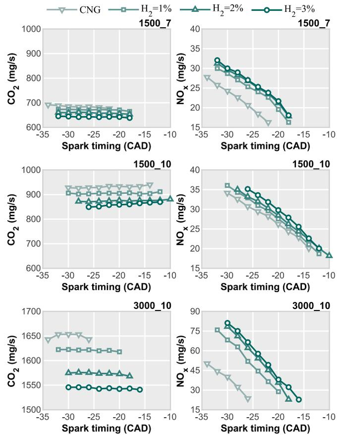
Fig. 5. NO<sub>x</sub> and CO<sub>2</sub> exhaust mass flow measurements.
