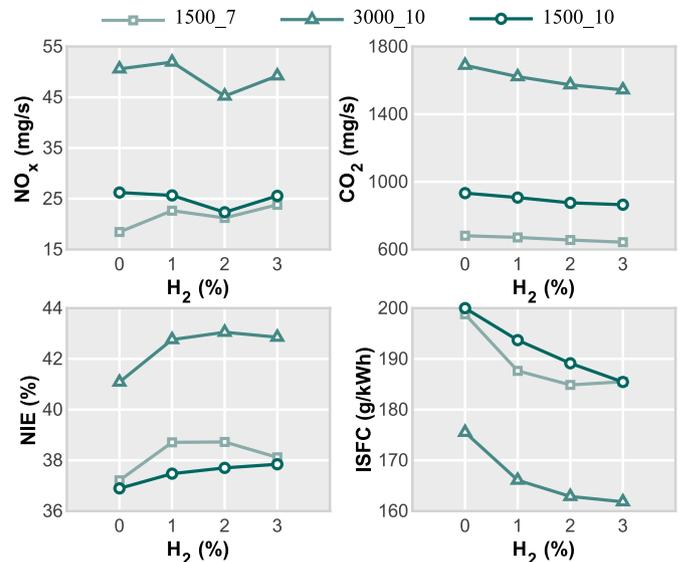
Fig. 6. Emissions (CO<sub>2</sub> and NO<sub>x</sub>) and performance (NIE and ISFC) for different operating points and fuel compositions.
