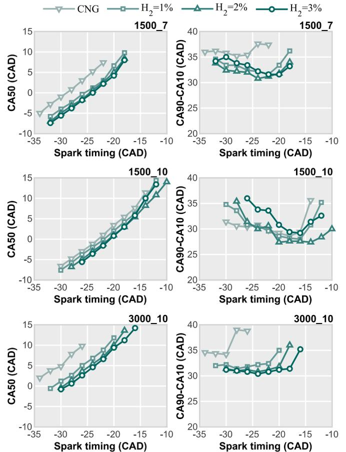
Fig. 3. Combustion phasing (CA50) and Combustion duration (CA90-CA10) for different hydrogen substitution percentages for different spark timing values.
