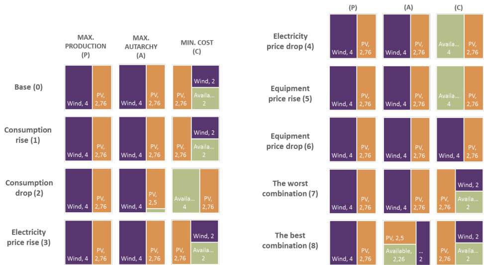
Figure 3.4.5: PV and Wind power (MW) for each sensitivity analysis alternative.
