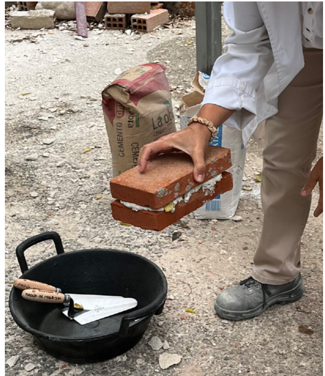
Figure 2. Adherence between two bricks in horizontal position (Image by the authors).
