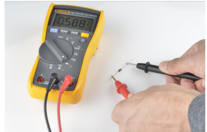
A multimeter with a diode setting can be used to measure (the minimum of) a diode's forward voltage drop.
