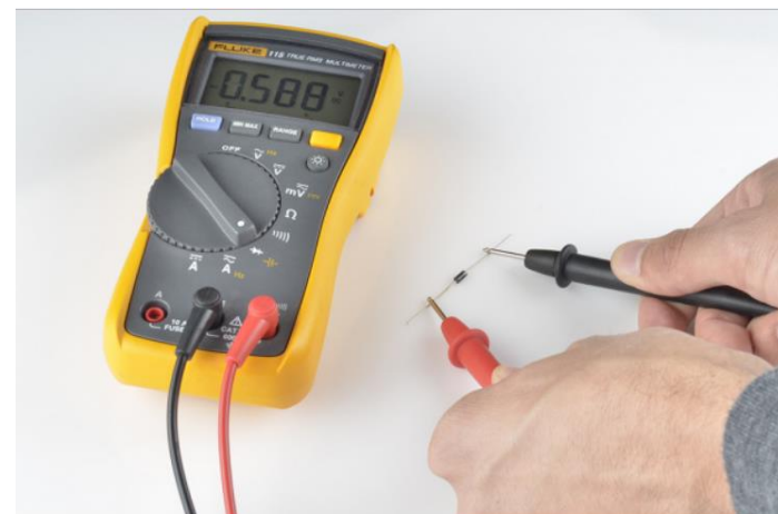
A multimeter with a diode setting can be used to measure (the minimum of) a diode's forward voltage drop.
