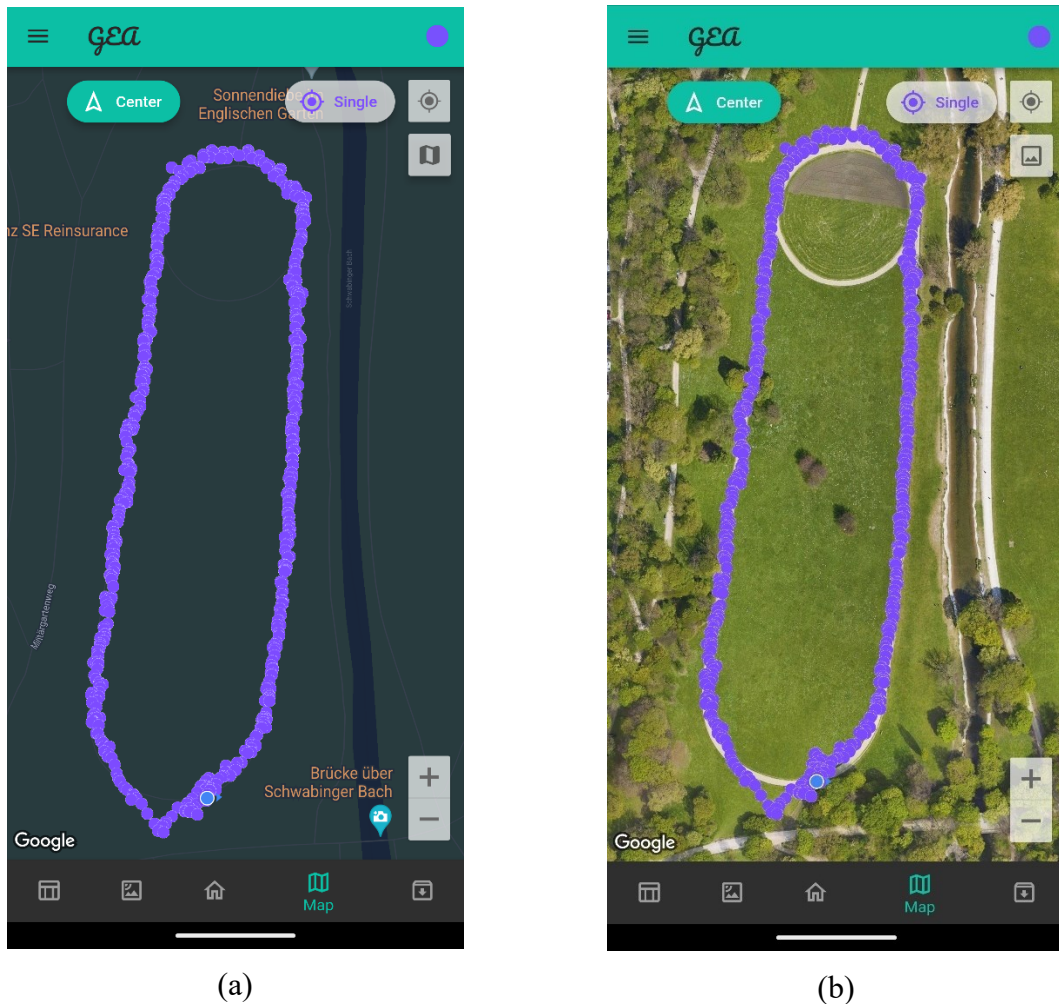
Figura 9: Positioning solution. (a) Map tab illustrating the position overlaid on a cartographic layer. (b) Map tab displaying the position superimposed on an aerial orthophotograph. Maps generated using GEA application version 2.1.0.
