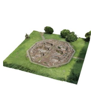
Figure 15. Photogrammetric data of the Baths: a) dense point clouds, b) mesh and (c) textured models.
