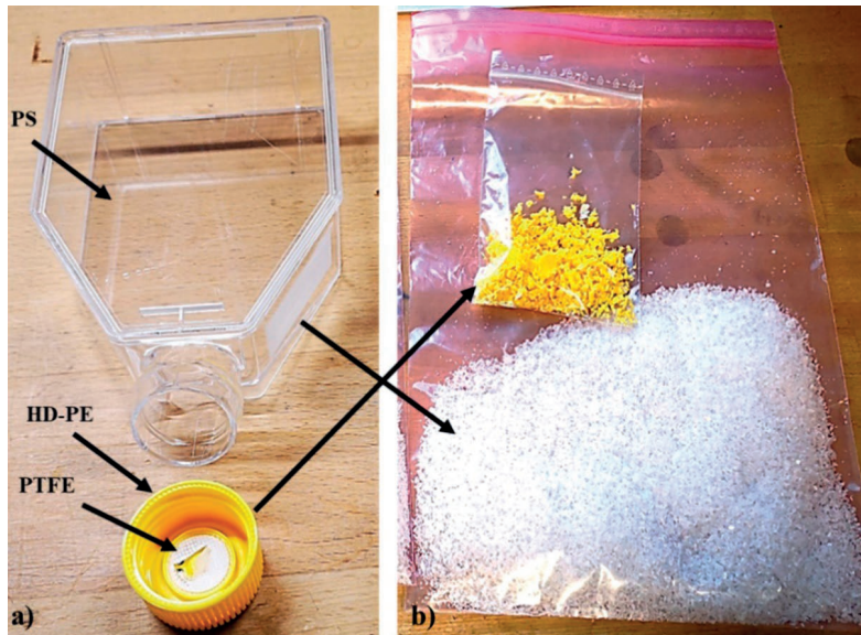
Figure 2. Cell culture flask, components and materials (a) and granulated components (b).
