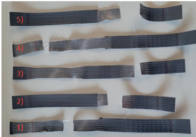
Figure 5. Samples of the Bauder Thermofol stored at room temperature after breakage.
