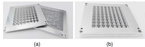
Fig. 7. Manufactured prototype. (a) Cover slipped and (b) full assembly.
