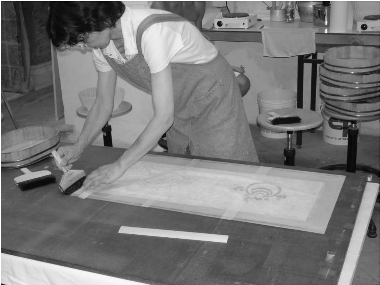
Figure 3. Preparing a sheet for tension flattening on a karibari. The karibari is a purpose-built base for paper tension flattening. This base is a traditional tool of Japanese papermakers which has been successfully adapted for its use in paper conservation
