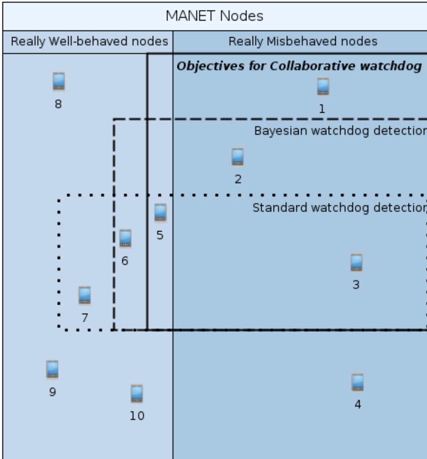
Figure 3.3: Graphical representation of the evaluation objectives for the Collaborative Bayesian Watchdog.
