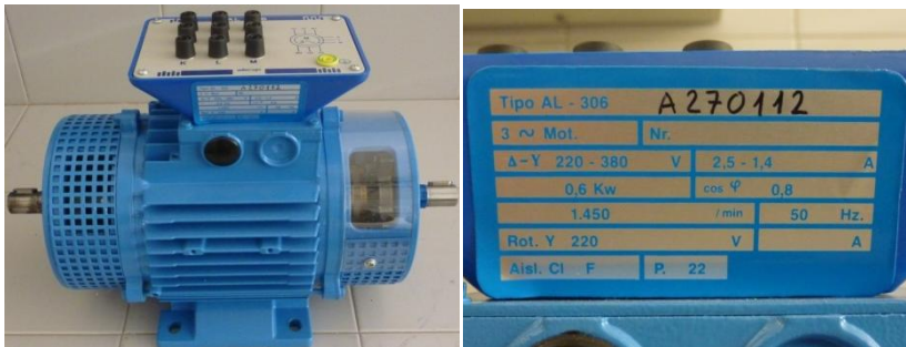
Fig. 201 600 W wound rotor induction machine and its nameplate.
