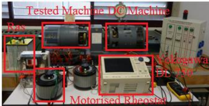
Fig. 65 Picture of the test bed for the test of the universal machine, set as wound rotor induction machine, in non-stationary stochastic conditions for the rotor asymmetry fault.
