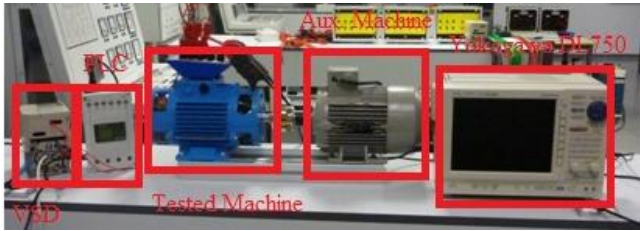
Fig. 170 Picture of the test bed for the test of the wound rotor induction machine with a mixed eccentricity
