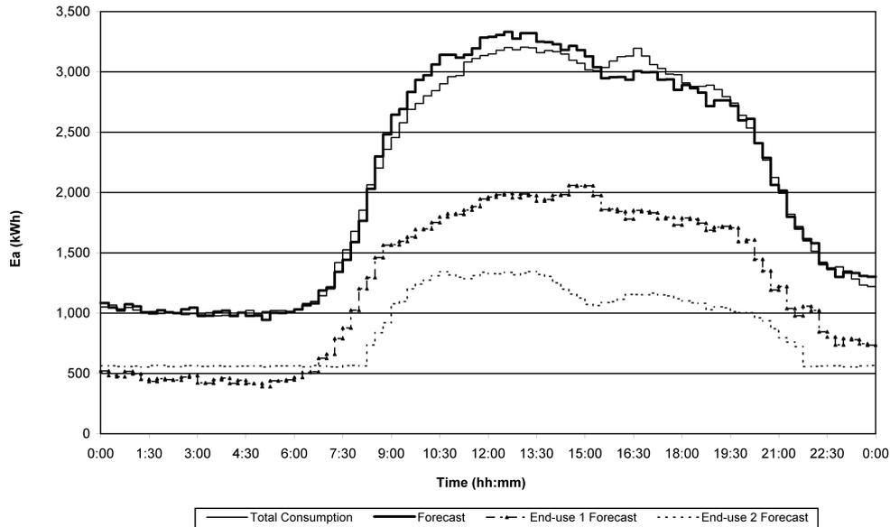
Figure 7. UPV consumption forecast for 25/06/2007 using EUs method.
