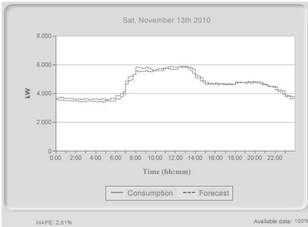
Figure 6. UPV consumption forecast implementation obtained on a Web platform.
