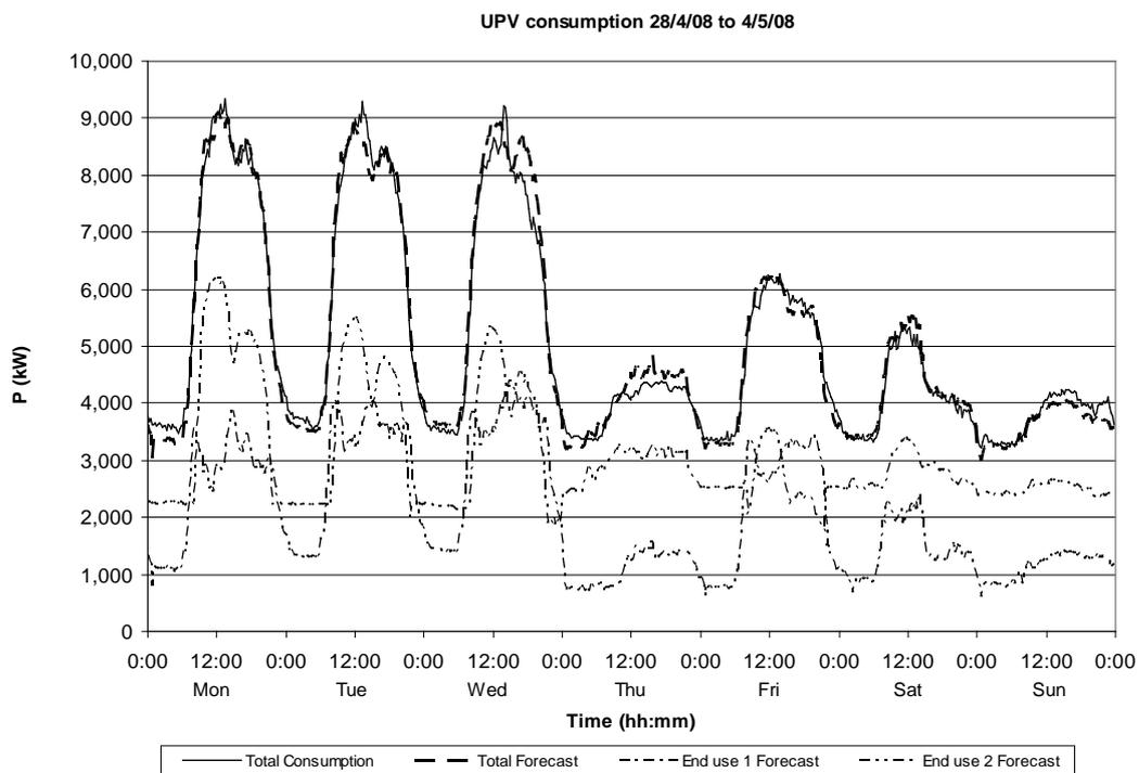
Figure 8. UPV consumption forecast for 28/04/08 to 04/05/08 using EUs method.
