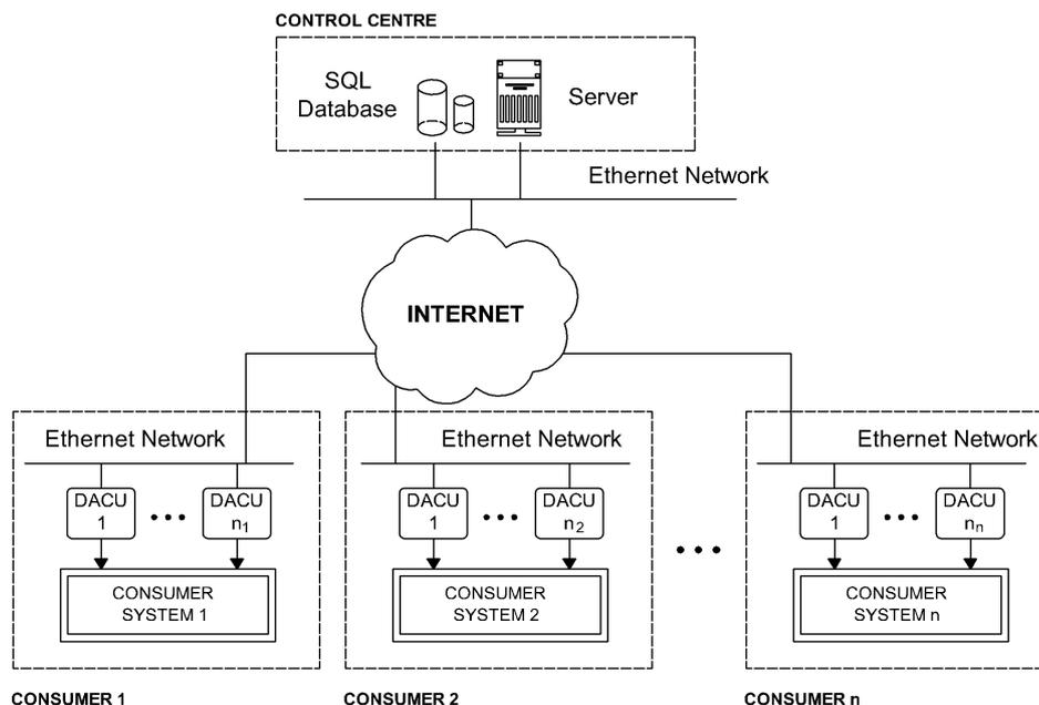
Figure 4. Recommended data acquisition architecture.
