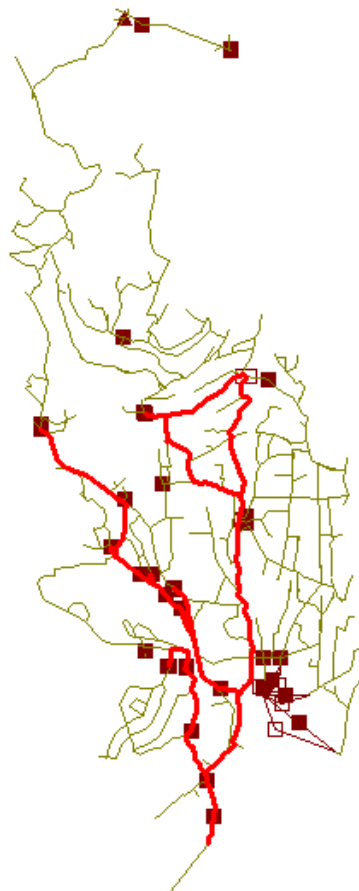
A total of 37 pipe groups were used as a starting point to run the optimisation
