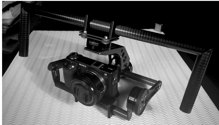
Figure 7. Gimbal 1 for bigger cameras in helicopters
