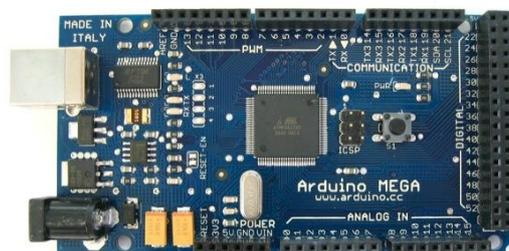
**Figura 3.20.** Arduino Mega 2560.
