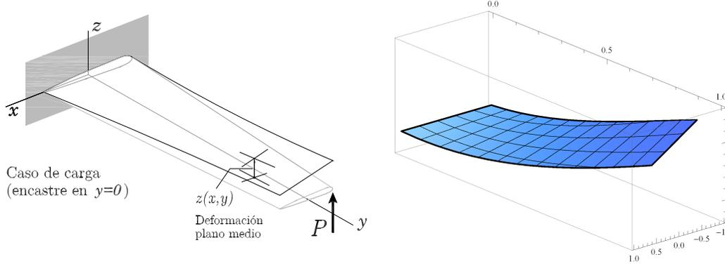
Figure 4: Elastic deformation due to an eccentric point-load at wingtip. Load case (left) and wing middle-plane deformed, calculated with Mathematica (right)
