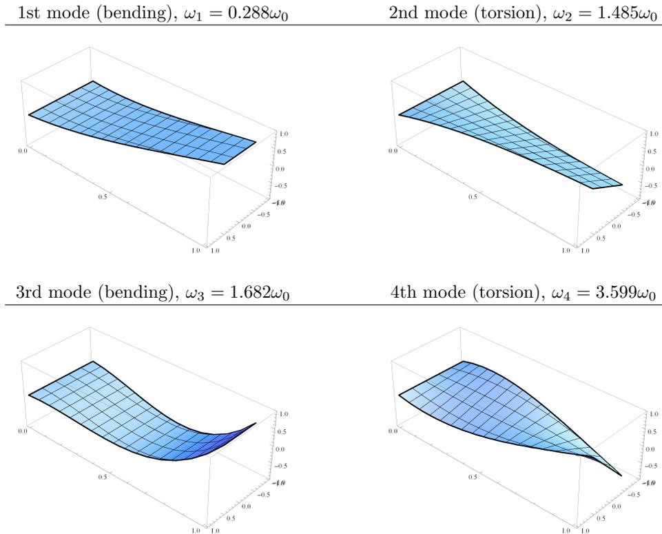
Figure 6: Undamped on-ground vibrating modes and associated natural natural frequencies referred to  $\omega_0 = \sqrt{GJ/mb_0^3}$  for  $EI = 0.9GJ$  and  $l = 6b_0$
