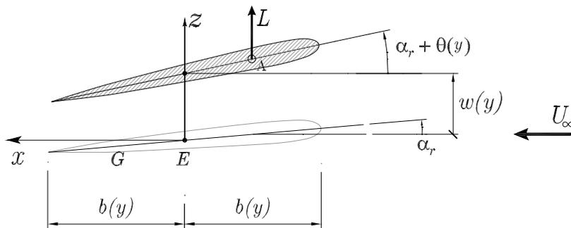
Figure 5: Rigid and elastic rotation angle of a arbitrary airfoil located at  $y = \eta l$ .
