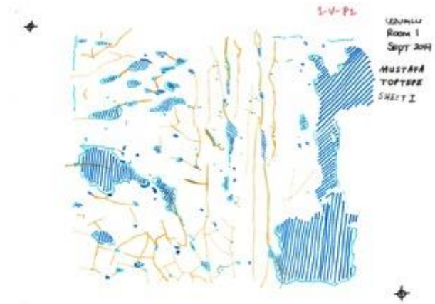
Figure 16: Scanned OHP sheet of plaster deterioration on the ceiling in narthex.
