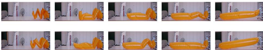
Figure 14. Folding sequence of deployable Tensairity beam with foldable truss mechanism
