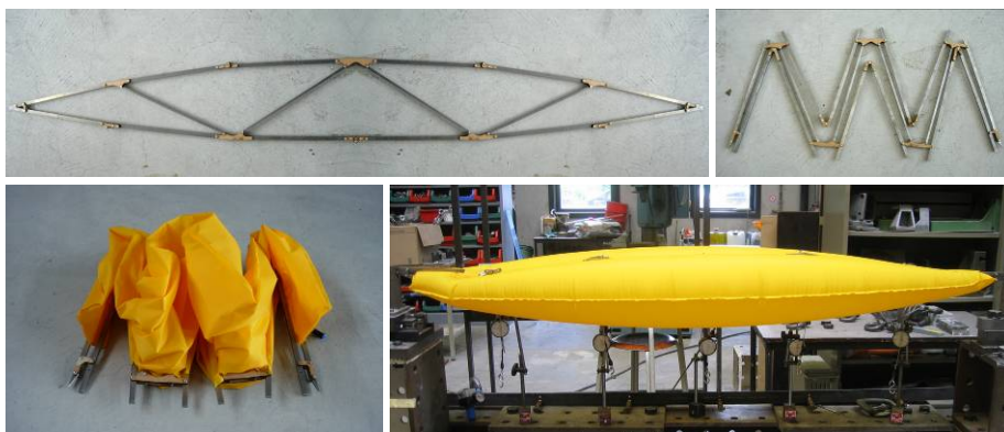
Figure 19. Investigations on a spindle shaped deployable Tensairity beam
