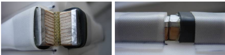
Figure 5. Detail of ‘segmented compression element’ – folded and unfolded
