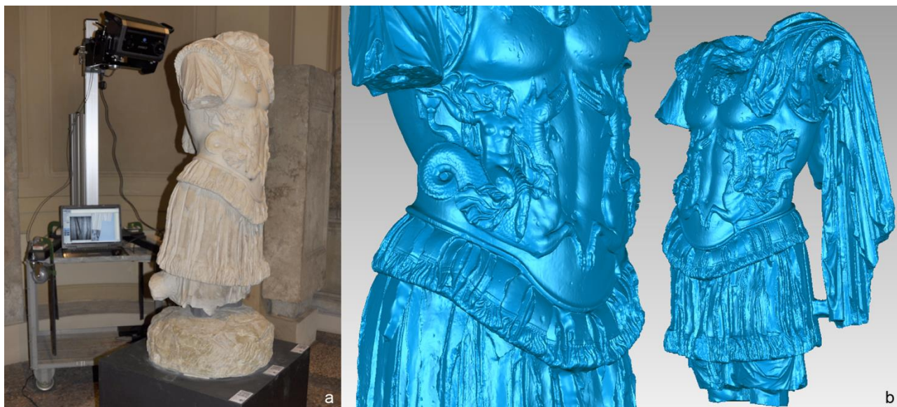
Figure 5: a) On site survey of the torso using a Konica Minolta Range 7 laser scanner; b) Views of the decimated 3D model (up to 25 million polygons).
