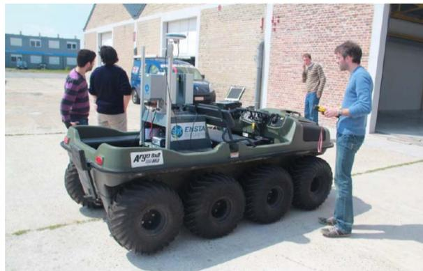
**Figure 5:** The used amphibious vehicle ARGO with equipment
