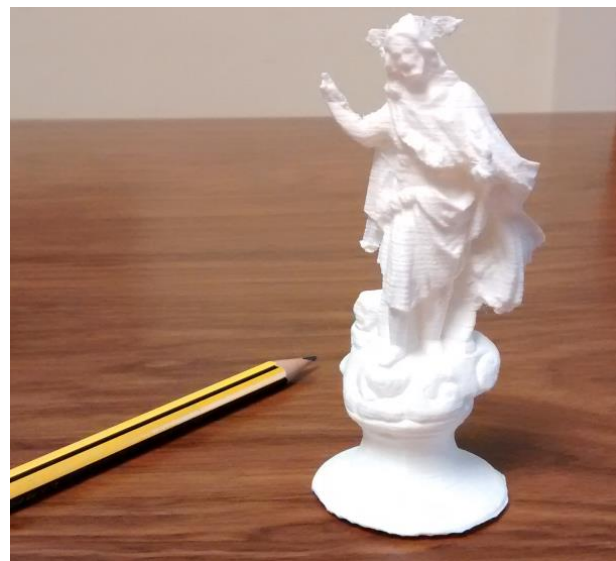
Figure 9: 3D printed model of the replica. A few elements, such as the banner or parts of the crown, were neglected during the scanning process because of the printer resolution. The figure has a height of 70 mm.
