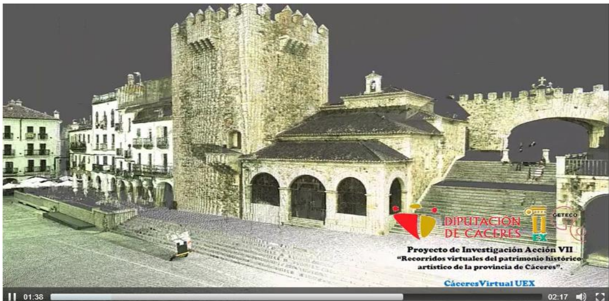
Figure 16: Video obtained from the point clouds measured by TLS.
