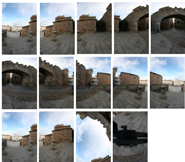
Figure 6: Images captured with the camera to generate a photograph (12 horizontal photographs, one zenith and another towards the ground).
