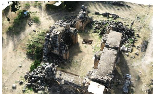
Figure 17: A 3D view of the textured DSM processed from the Terme-Chiesa flight.
