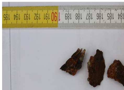
Fig. 8- Through hole's residues ferrous of fig.7
