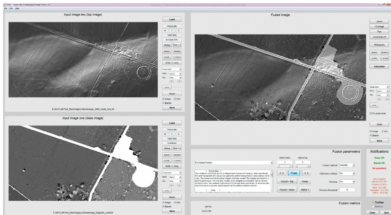
Figure 2: The main TAIFU window. A digital terrain model (upper left) is fused with a magnetogram (lower left) using ICA-based fusion.
